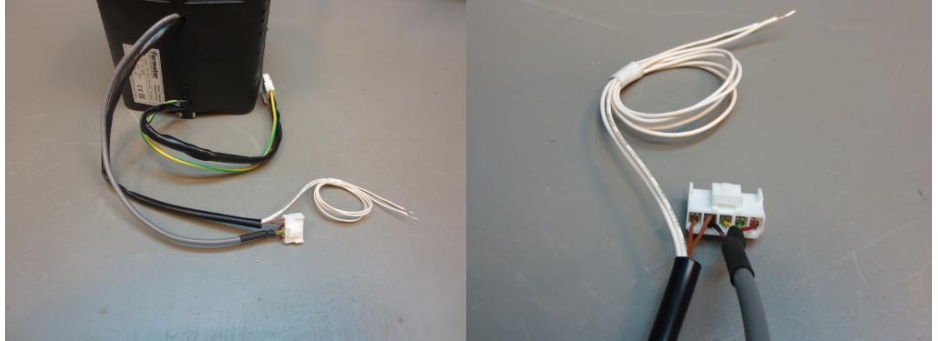
Picture 11: Main Motor VF with Thermal Sensor and Encoder.
